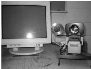
Figure 2. An ISCAN, Inc. remote video-based eyetracker, set up for recording movements of one or the other eye during viewing of simple scenes on a computer screen. The cylinder in between the monitor and the camera lens is the infrared emitter. The mechanism immediately below the camera itself allows it to tilt up and down and pan left and right to accommodate small head movements.
