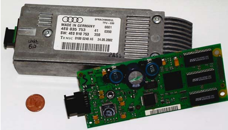
Figure 1. Hardware speech dialogue module.
